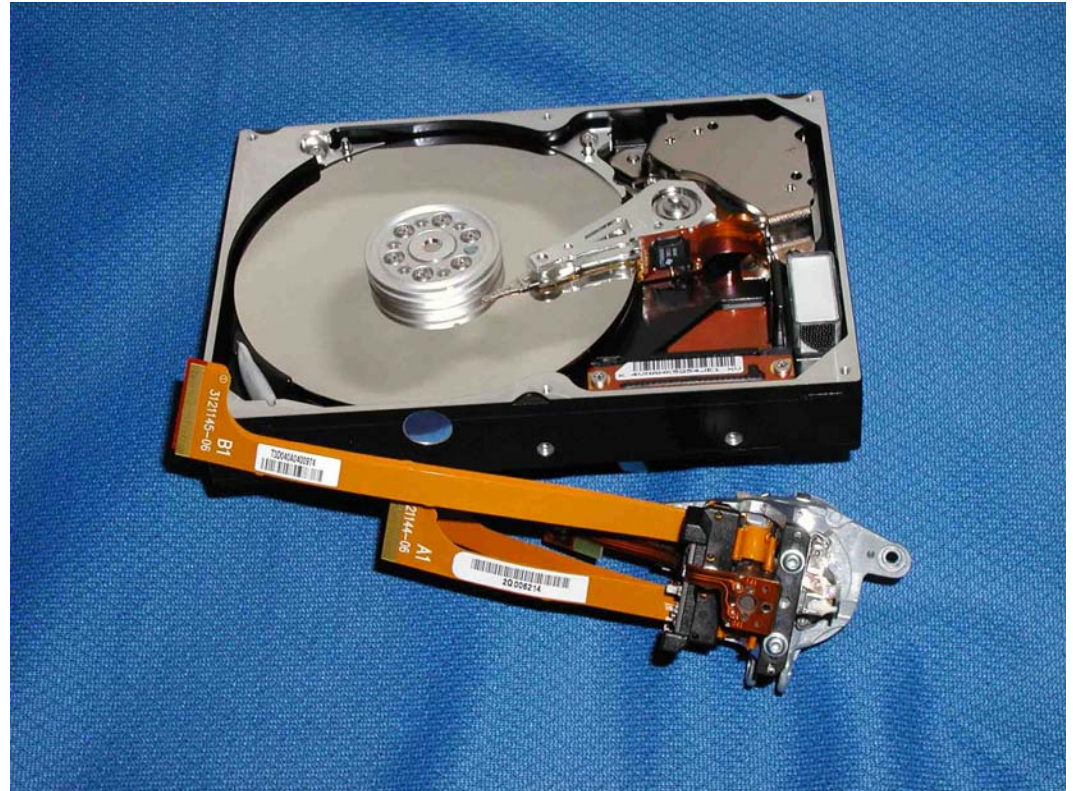
2006 Maxtor hard drive Sun T10000 head, flex, and voice coil
